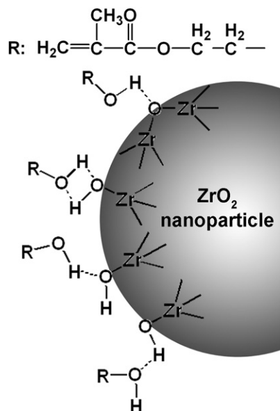
Scheme 1. Possible fashion of hydrogen bond between HEMA and ZrO_2 nanoparticles.
